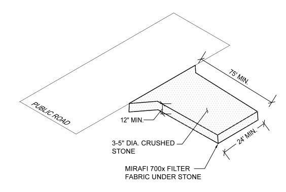
CONSTRUCTION EXIT DETAIL NOT TO SCALE
