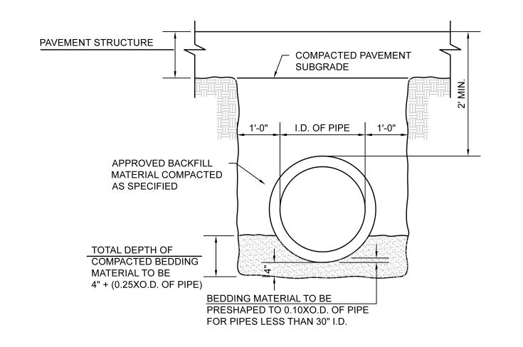
STORM SEWER TRENCH DETAIL NOT TO SCALE
