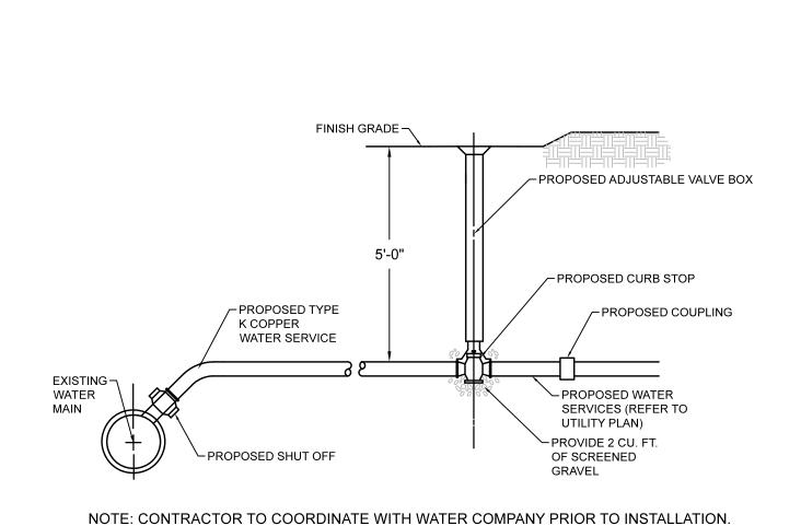
WATER SERVICE CONSTRUCTION DETAIL NOT TO SCALE
