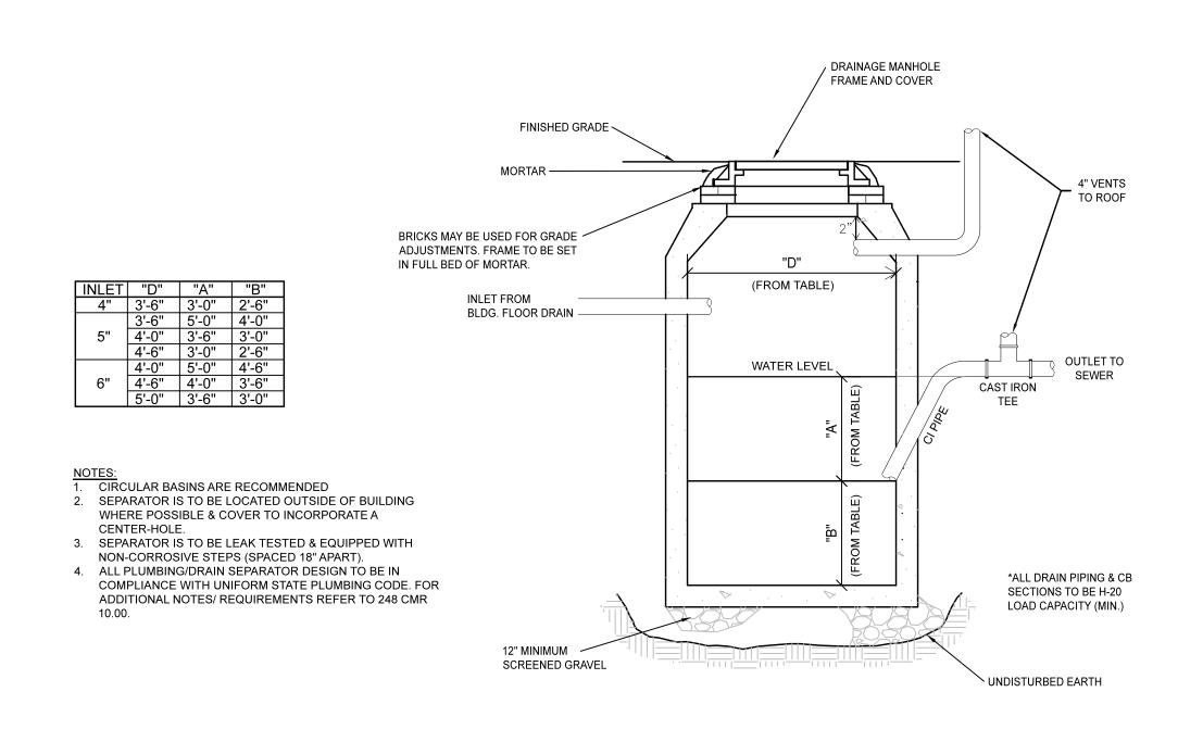
TYPICAL OIL/ GREASE SEPARATOR DETAIL NOT TO SCALE
