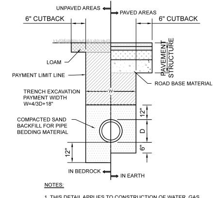
1. THIS DETAIL APPLIES TO CONSTRUCTION OF WATER, GAS, TELEPHONE, ELECTRIC, AND CABLE TELEVISION UTILITIES. UNLESS DIRECTED OTHERWISE BY APPLICABLE UTILITY COMPANIES. 2. PROVIDE 5' MINIMUM COVER OVER WATER SERVICE LINE UNLESS DIRECTED OTHERWISE BY WATER COMPANY.
