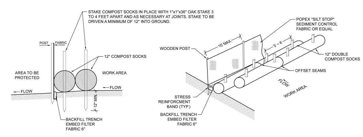
DOUBLE COMPOST SOCKS WITH SILT FENCE DETAIL NOT TO SCALE
