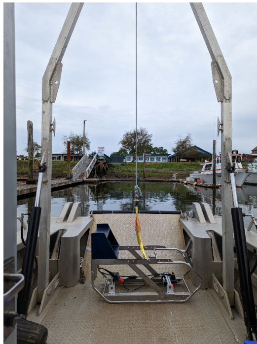
Photograph 10. Vessel for completing the macrovegetation surveys shown with towed underwater camera on deck of vessel. (June 15, 2022)
