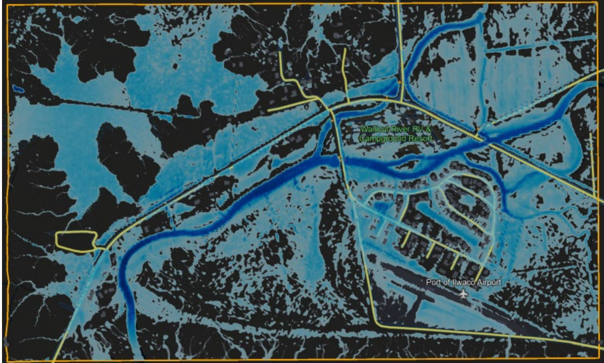
Figure 23. Flooding in the Vandalia Focus Area in a back water situation with 3-10ft culverts under Stringtown Rd.
