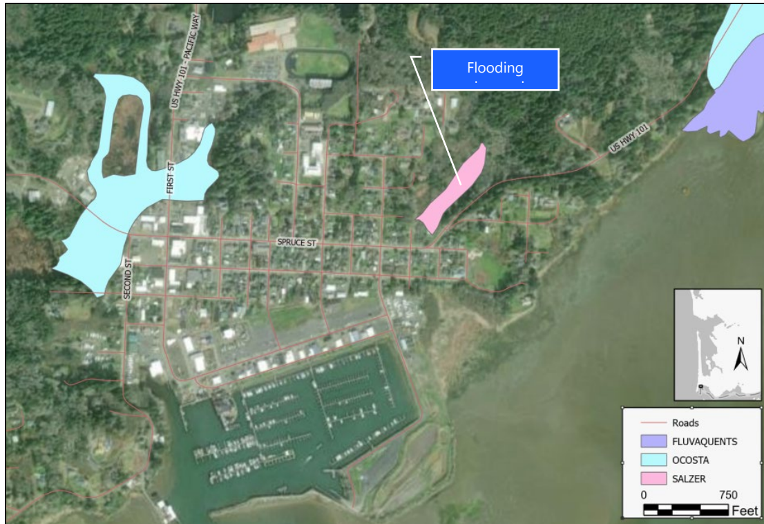
Figure 8. The presence of low-permeability soils in the City of Ilwaco focus area. Flooding is observed at the marker during King Tides due to backflow effect up outfall pipe.
