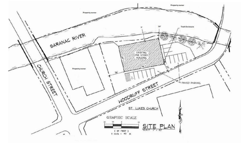
**Site Plan Checklist:** This sample plan is for reference only. Your plan may require additional information Property boundaries with setbacks, plotted to scale Location, width and name of a
