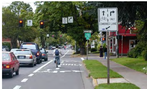
Shared bicycle/right turn lanes require warning signage as well as pavement markings
