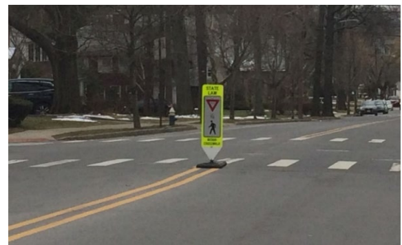
Signage Example – In Street flexible Yield to Pedestrian sign with base – Sign# R1-6d
