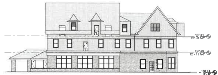
4 SURVEY ELEVATION - RIGHT 3/32" = 1'-0"
