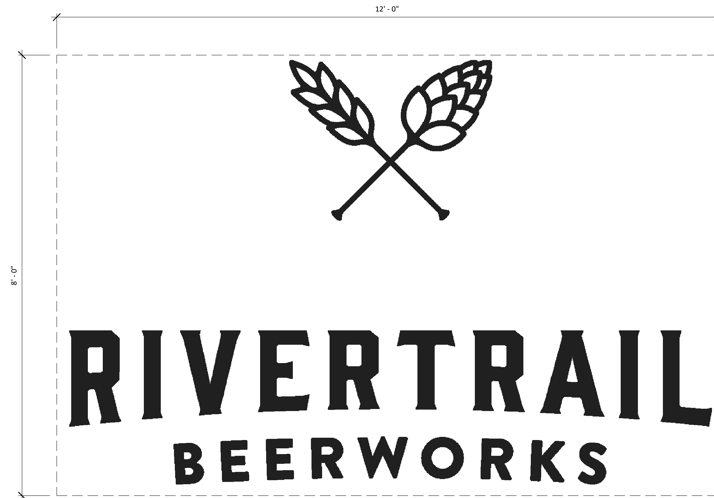
(1) PROPOSED WALL SIGNAGE: NORTH WALL -CUSTOM CUT WHITE LETTERING -12' X 8' X 1/2" (96 SF) -LIGHT WITH LED DARK SKY COMPLIANT GOOSENECK
