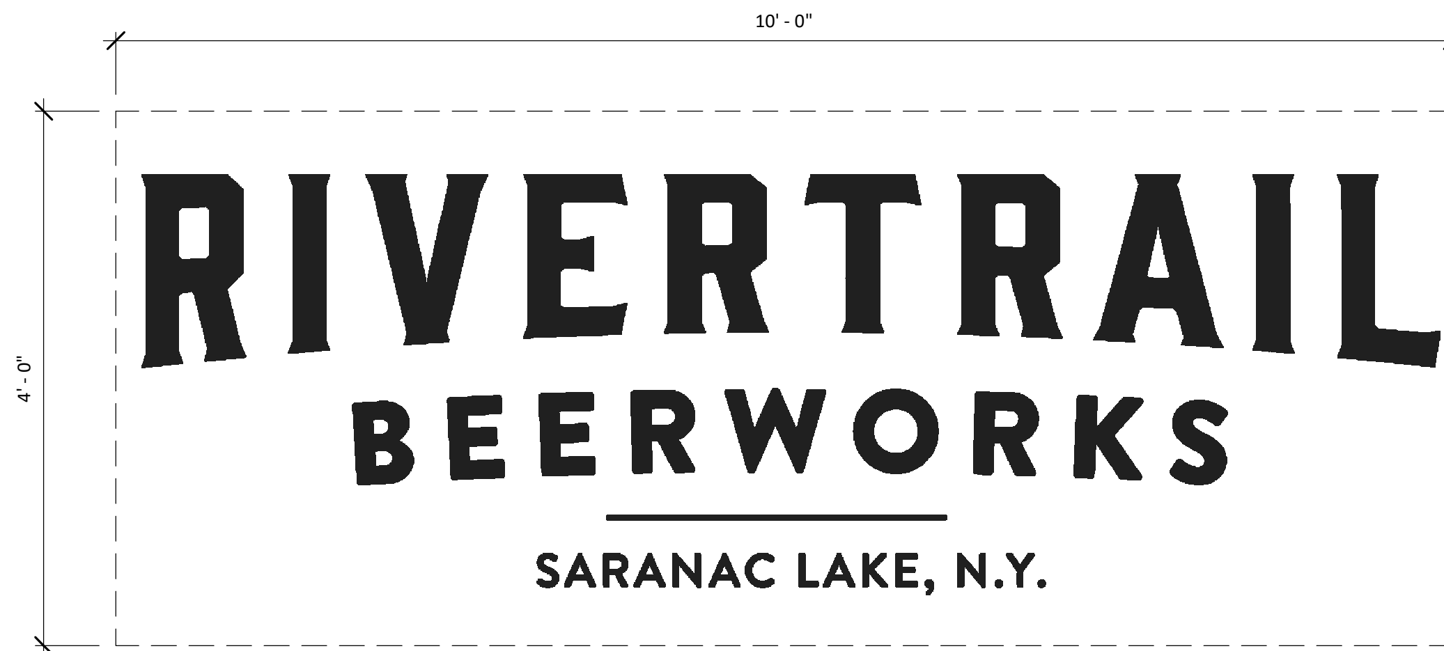
(2) PROPOSED GROUND SIGNAGE -16' T.O. LETTERING -CUSTOM CUT WHITE LETTERING -10' X 4' X 1/2" (40 SF) -INTERNAL LED LIGHTING
