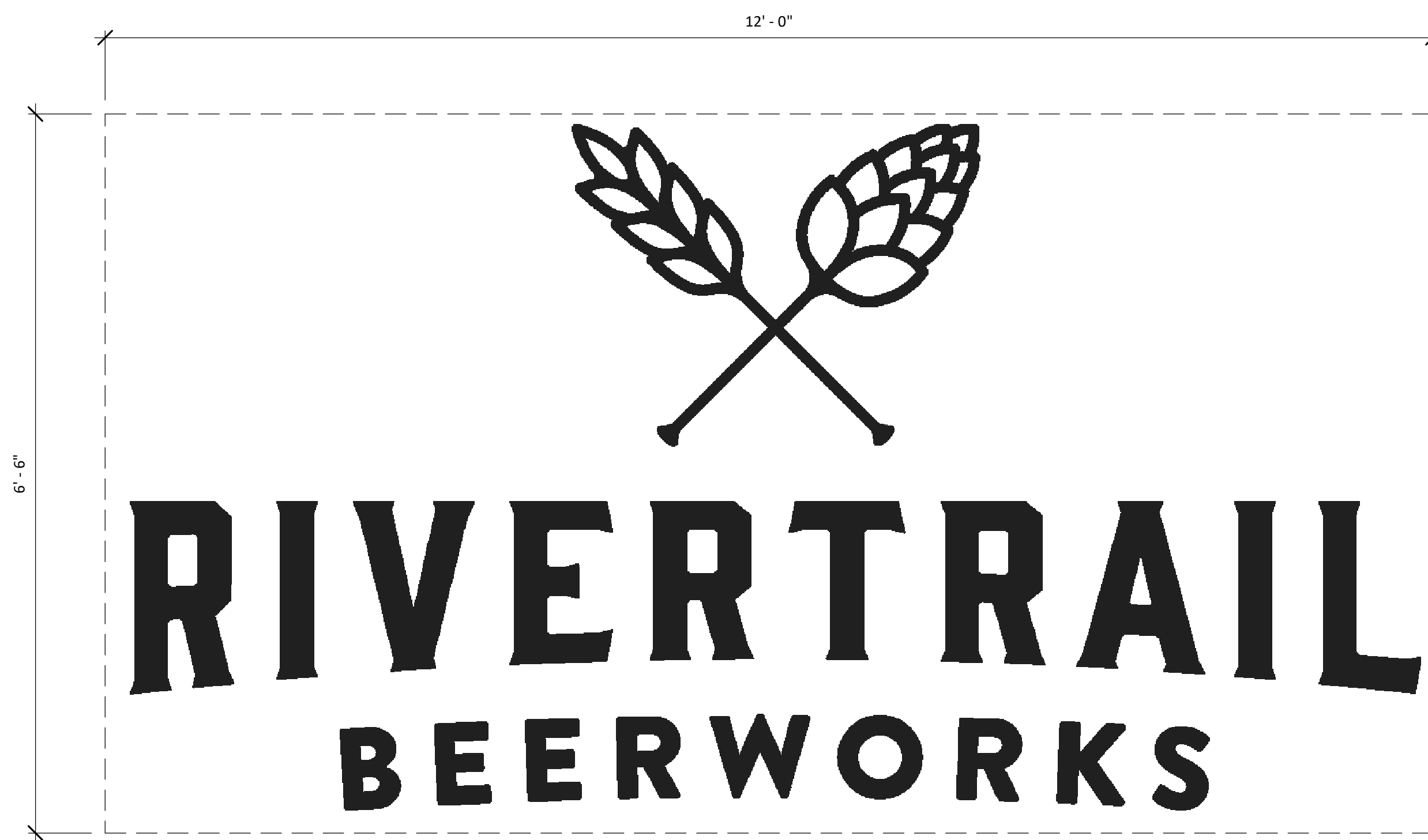
(1) PROPOSED WALL SIGNAGE: WEST WALL -CUSTOM CUT WHITE LETTERING -12' X 6'-6" X 1/2" (78 SF) -LIGHT WITH LED DARK SKY COMPLIANT GOOSENECK
