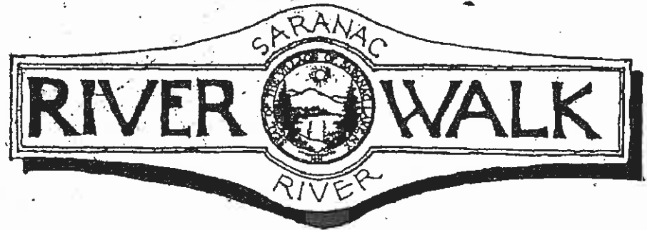
River walk identification sign made of aluminum with relief lettering and three color paint scheme. Locate on posts and wall corners along the walk.
