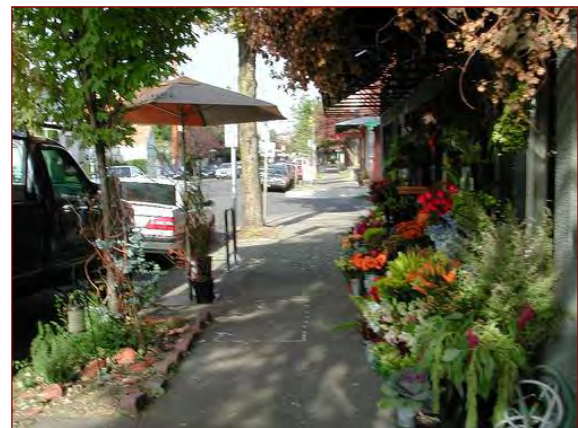
This sidewalk has plantings in the furnishing zone and in the frontage zone and provides sufficient through passage zone width
