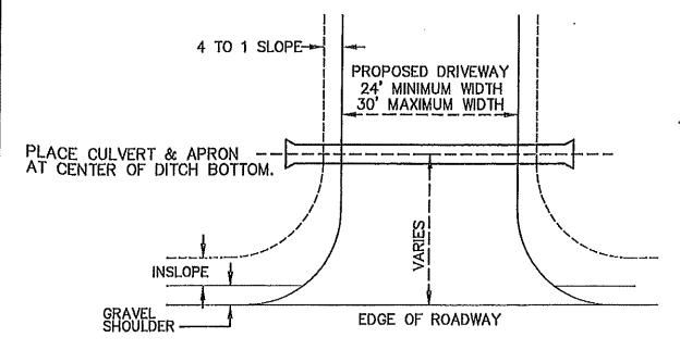
NOTES: CULVERT APRON LIP IS TO BE PLACED AT DITCH BOTTOM. IN THE OCCURRENCE THAT DITCH IS DEEPER THAN THE MINIMUM, THE CULVERT LENGTH SHALL BE EXTENDED TO MAINTAIN 4 TO 1 SLOPE.
