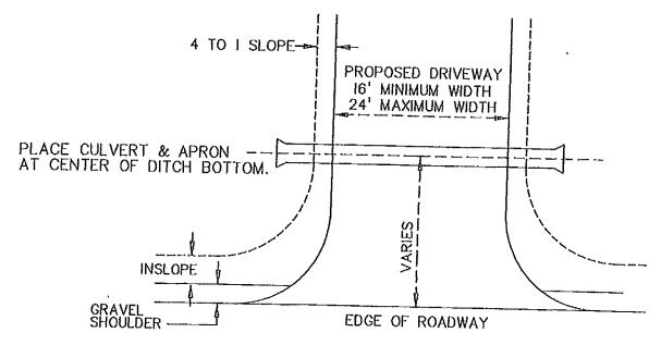
NOTES: CULVERT APRON LIP IS TO BE PLACED AT DITCH BOTTOM. IN THE OCCURRENCE THAT DITCH IS DEEPER THAN THE MINIMUM, THE CULVERT LENGTH SHALL BE EXTENDED TO MAINTAIN 4 TO I SLOPE.
