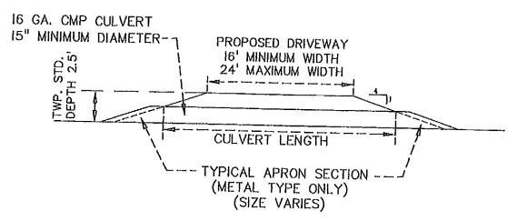
CULVERT LEN. (ft.) = DRIVEWAY WID. (ft.) + 2[((DITCH DEPTH-CULVERT DIA. in.)/i2) \* 4] EXAMPLE: I6 ft DRIVEWAY WIDTH, 29" DITCH DEPTH, I5" CULVERT CULVERT LEN. (ft.) = 16' + 2[((29"-15")/12) \* 4] = 25 ft.
