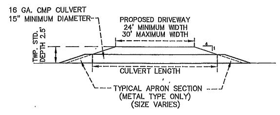
CULVERT LEN. (ft.) = DRIVEWAY WD. (ft.) + 2[((DITCH DEPTH-CULVERT DIA. in.)/12) \* 4] EXAMPLE: 16 ft DRIVEWAY WIDTH, 29" DITCH DEPTH, 15" CULVERT CULVERT LEN. (ft.) = 24' + 2[((29" - 15")/12) \* 4] = 33 ft.
