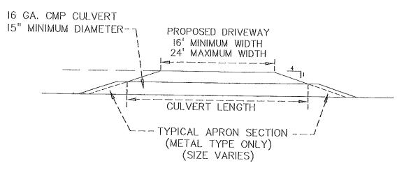
CULVERT LEN. (ft.) = DRIVEWAY WID. (ft.) + 2[((DITCH DEPTH-CULVERT DIA. in.)/I2) \* 4] EXAMPLE: I6 ft DRIVEWAY WIDTH, 29" DITCH DEPTH, I5" CULVERT CULVERT LEN. (ft.) = 16' + 2[((29"- 15")/I2) \* 4] = 25 ft.
