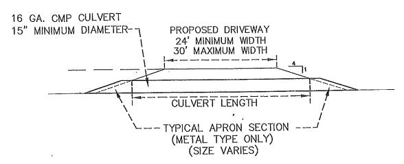
CULVERT LEN. (ft.) = DRIVEWAY WID. (ft.) + 2[((DITCH DEPTH-CULVERT DIA. in.)/12) \* 4] EXAMPLE: 16 ft DRIVEWAY WIDTH, 29" DITCH DEPTH, 15" CULVERT CULVERT LEN. (ft.) = 24' + 2[((29'' - 15'')/12) \* 4] = 33 ft.
