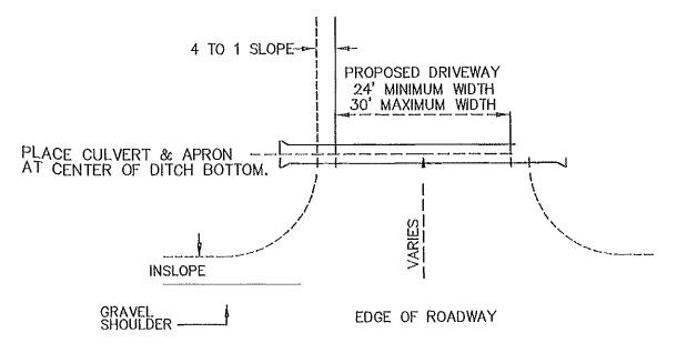
NOTES: CULVERT APRON LIP IS TO BE PLACED AT DITCH BOTTOM. IN THE OCCURRENCE THAT DITCH IS DEEPER THAN THE MINIMUM, THE CULVERT LENGTH SHALL BE EXTENDED TO MAINTAIN 4 TO 1 SLOPE.
