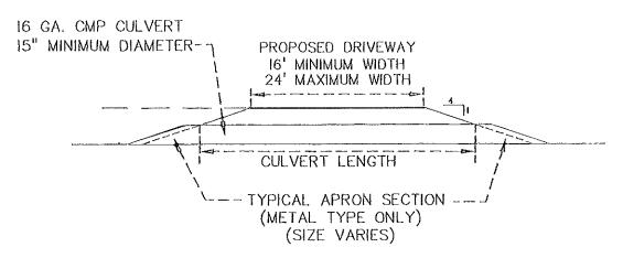
CULVERT LEN. (ft.) = DRIVEWAY WID. (ft.) + 2[((DITCH DEPTH-CULVERT DIA. in.)/12) \* 4] EXAMPLE: 16 ft DRIVEWAY WIDTH, 29" DITCH DEPTH, 15" CULVERT CULVERT LEN. (ft.) = 16' + 2[((29"- 15")/12) \* 4] = 25 ft.
