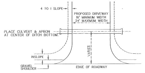
NOTES: CULVERT APRON LIP IS TO BE PLACED AT DITCH BOTTOM. IN THE OCCURRENCE THAT DITCH IS DEEPER THAN THE MINIMUM, THE CULVERT LENGTH SHALL BE EXTENDED TO MAINTAIN 4 TO I SLOPE.
