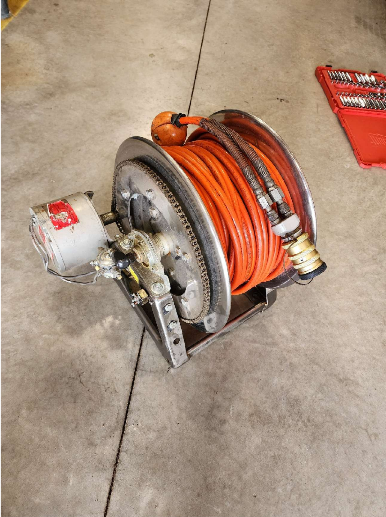
(F) 12V hose reel with Hydraulic hose and quick connect fittings
