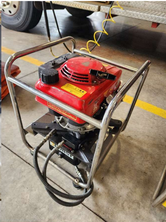
(A) Honda GXV120 Motor with HURST hydraulic power unit.
