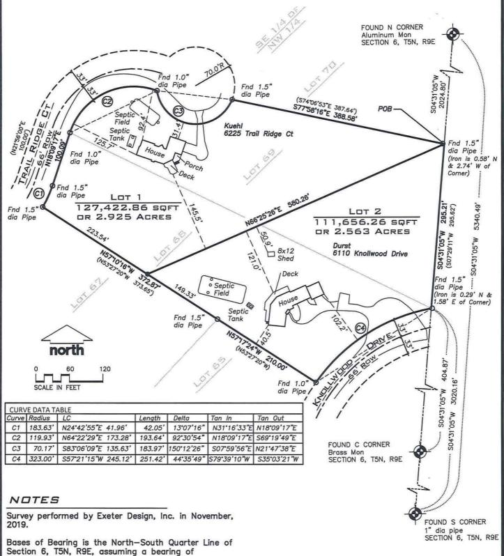
Bases of Bearing is the North-South Quarter Line of Section 6, T5N, R9E, assuming a bearing of S04\*31'05"w.
