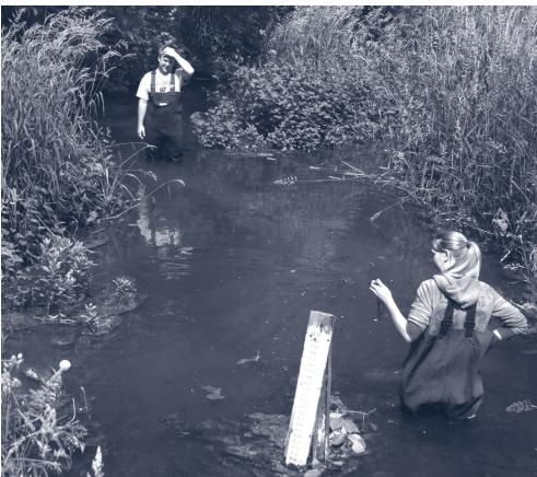
Dylan Kersten (left), Miranda Heimstreet (right) and Jeanne Scherer (photographer) take water quality measurements at the inlet and outlet to Lake Ripley. Here they're seen timing the stream's flow rate.
