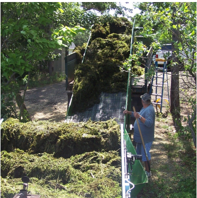
A load of plants is offloaded from the harvester into the shore conveyor. Material is then loaded into a dump truck carried to a compost site.
