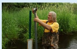
Jimmy DeGidio checks water levels on Lake Riplev's inlet stream. New equipment seen here is being deployed to help determine phosphorus inputs into the lake, so we can take steps to reduce that phosphorus.
