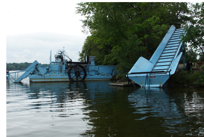
Lake Ripley's weed harvester and offload conveyor.
