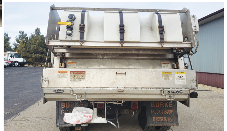
The brine tank is attached to the back of the truck. The brine mixture pre-wets the salt before the salt is spread on the roadways.
