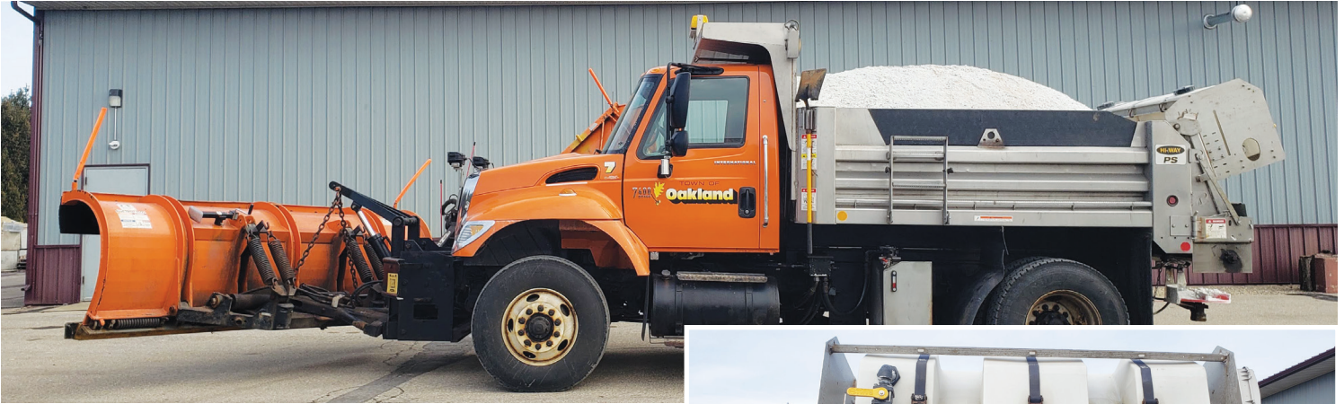
One of the snowplows Jeff and his team use. This plow has the brine tank on the back of it to pre-wet the salt.
