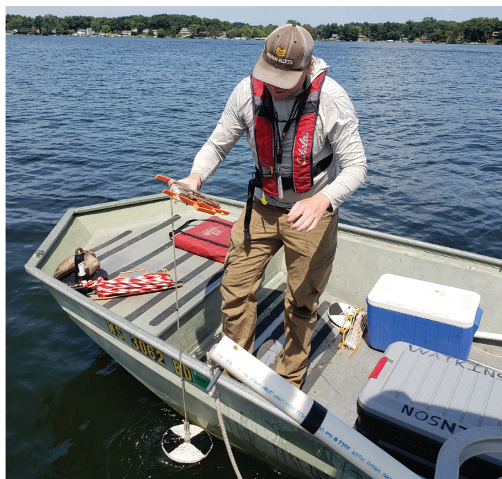
DNR's Arthur Watkinson measuring the clarity on Lake Ripley using a secchi disk.
