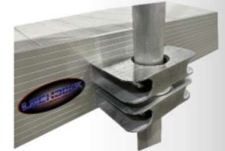
Floating Post Collars Are Typically At All Corners Of The System. Sometimes More Are Added On Bigger Systems. The Collars Have A 3" Nylon Bushing That The Oversized 2-3/8" Poles Move Against.
