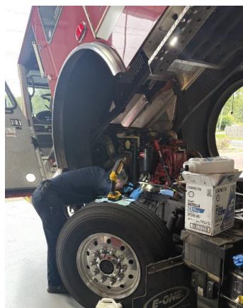
Firefighter Simon conducts oil and filter change on E101-repairs and preventative maintenance done in-house saves thousands of dollars each year and ensures our apparatus are ready to go at a moment's notice.
