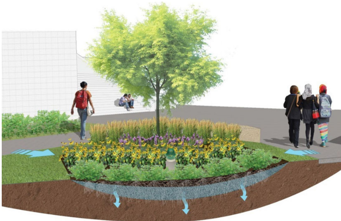
Figure 16: Bioretention basin diagram
