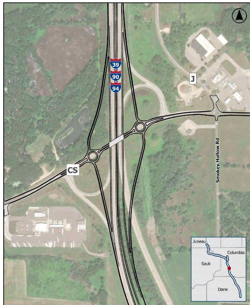
Figure F: WisDOT-Recommended Diamond Interchange at CTH CS
