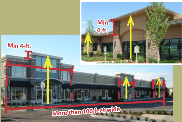
APPROPRIATE The images above illustrate techniques used to vary the facade heights along a long facade, meeting the 25% threshold described in Standard 3 .
