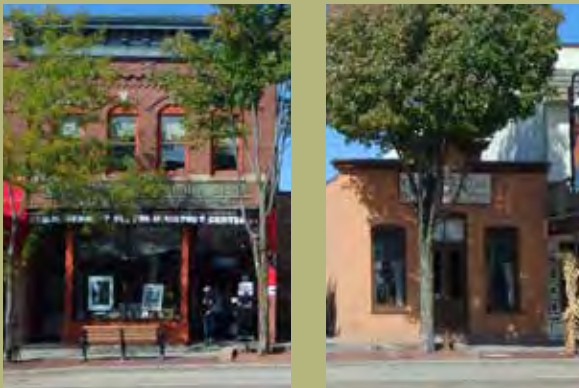
APPROPRIATE The above signage is placed in historical storefront locations (i.e. above the first floor windows/doors but below the second story sills, centered above the doorway, and along the awning profile).
