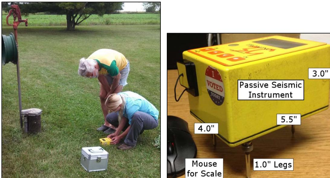
**Figure 3-1.** The Passive Seismic instrument shown in the field (left) and up close (right). The three 1-inch metal legs are inserted into the ground to record ambient ground vibrations. A computer mouse is shown for scale next to the instrument.
