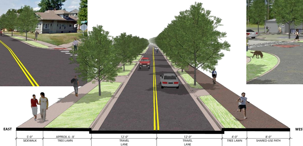
Cross-Section Looking South - Front Street Olean, NY
