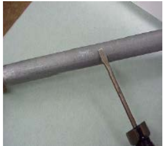
Galvanized Iron – dull steel color; magnet
