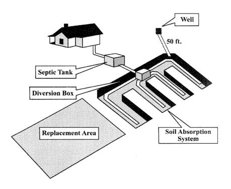
Absorption fields can fail in two ways: 1) they can fail to absorb the septic tank effluent, or 2) they can fail to treat the effluent by not filtering out parasites and pathogenic
