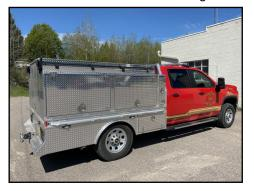
set it up, we opted for a high capacity suction ability pump to be able to transfer water from the many streams and lakes into tanker trucks when hydrant water is not feasible as a water source. We have had several trainings with this new unit and are very pleased with results. We can move 3000 gallons of water from a lake into a tanker truck in 7 minutes 11 seconds! 417 gallons a minute! For perspective, your kitchen faucet flows about
