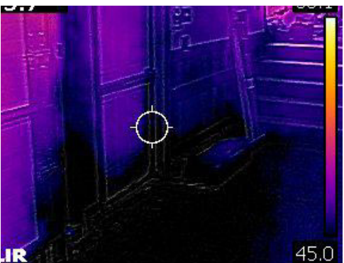
THERMAL SCAN AT APPARATUS BAY WALL #3: The floor at the door again illustrates the lack of insulation. In addition, the concrete sub-floor is cold inside the building. In the winter, as has been noted, that ice forms at inside portions of the building especially at the overhead doors and entrances. Under the floor tile, the slab is wet and prone to mold.
