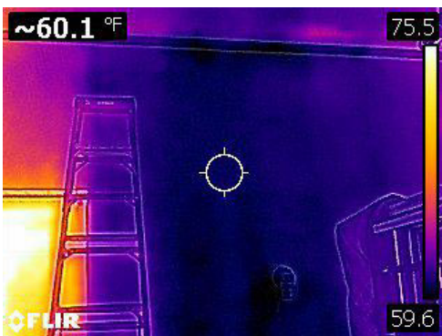
THERMAL SCAN AT APPARATUS BAY WALL #2: Here is another example of an exterior wall not insulated. The result is moisture and eventually mold within the wall cavity.
