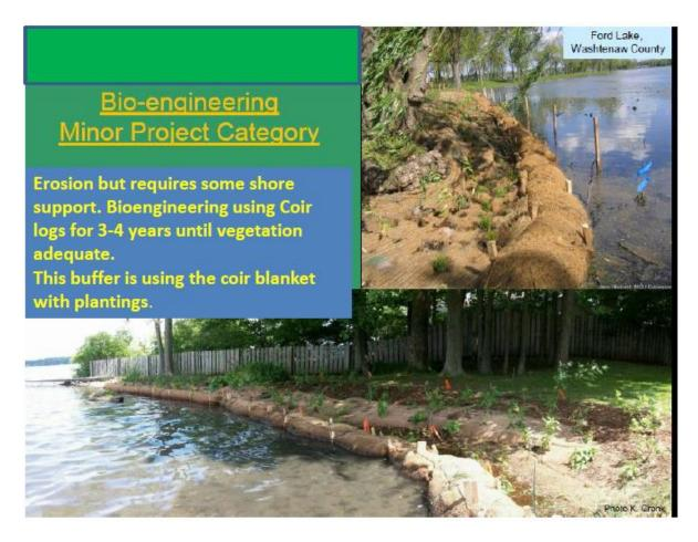
Soft engineering is using biologic material instead of or in combination with hardscape. Seawalls have been shown to cause damage to neighboring properties and break down frequently. Rip rap is expensive and if not installed according to marine engineering standards can also fail to protect the shore.
