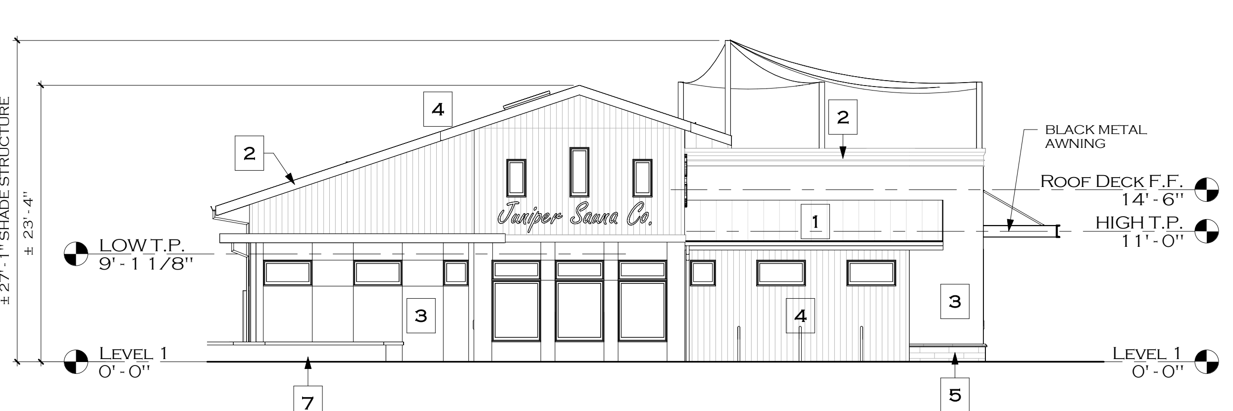
CLAY ST. SCALE: 1/8" = 1'-0" WALL AREA: 577.28 S.F. OPENINGS: 130.51 S.F. PERCENTAGE OF FACADE OPENINGS: 22.6%
