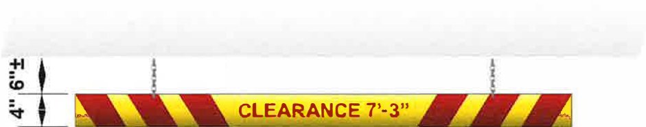
F FRONT ELEVATION @ TYPICAL HANGING CLEARANCE BOLLARDS SCALE: 3/4" = 1'-0" (3 REQ'D)
