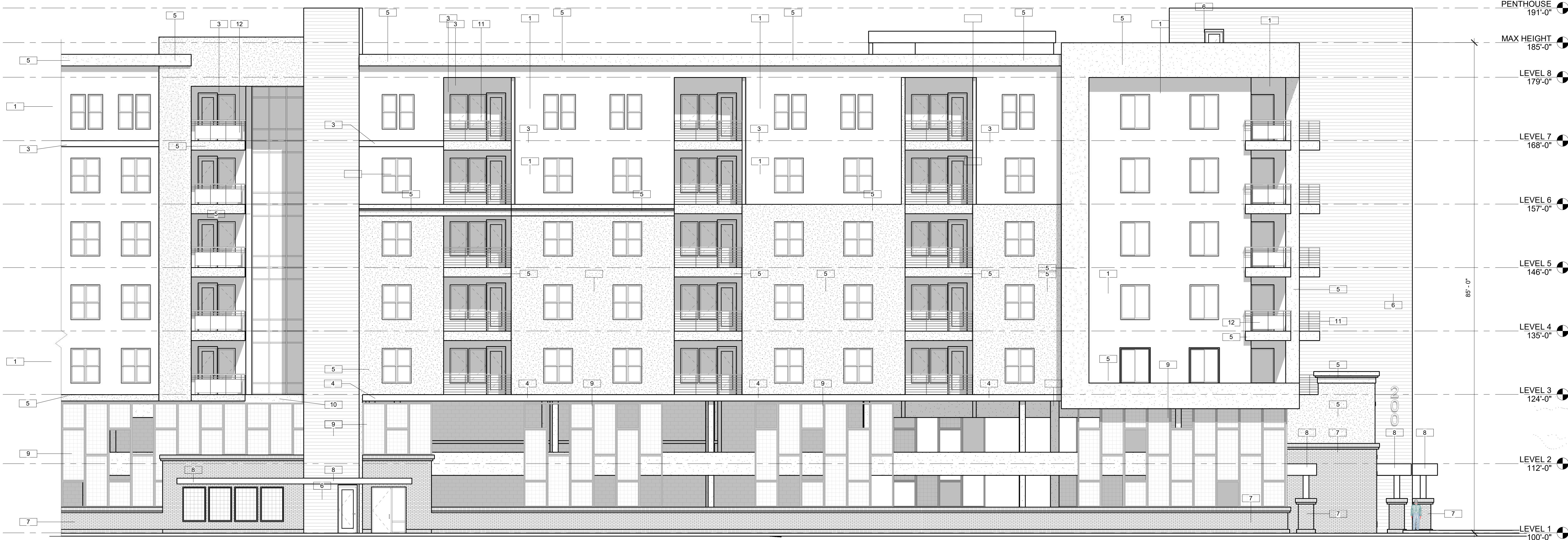
2 BUILDING ELEVATION - SOUTH-EAST 1/8" = 1'-0"
