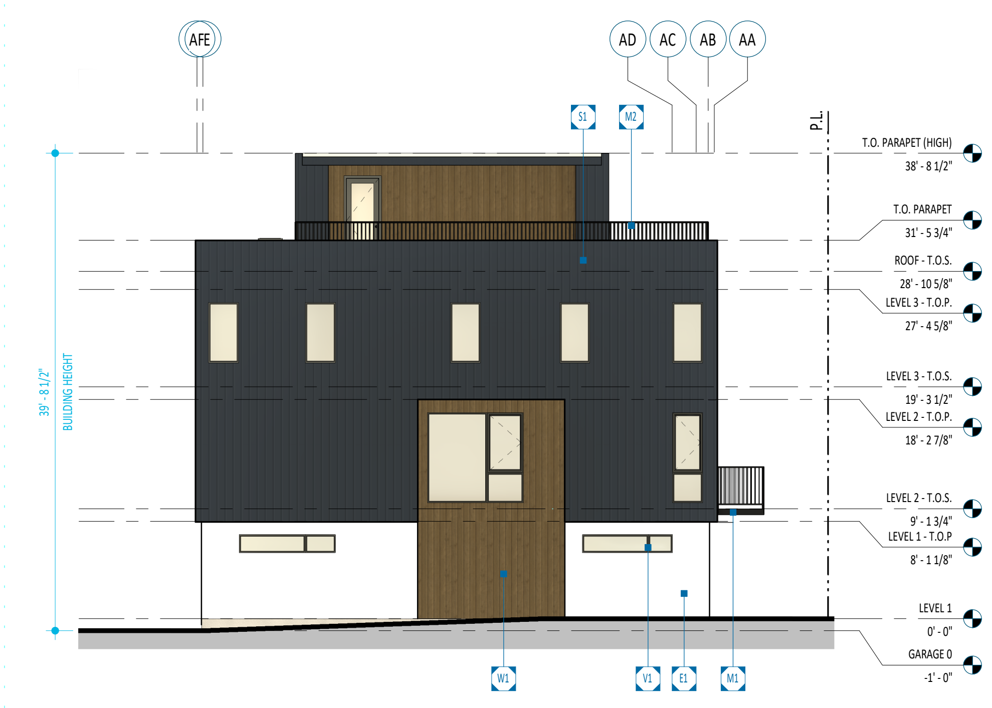
E1 EXTERIOR ELEVATION-EAST 1/8" = 1'-0"
