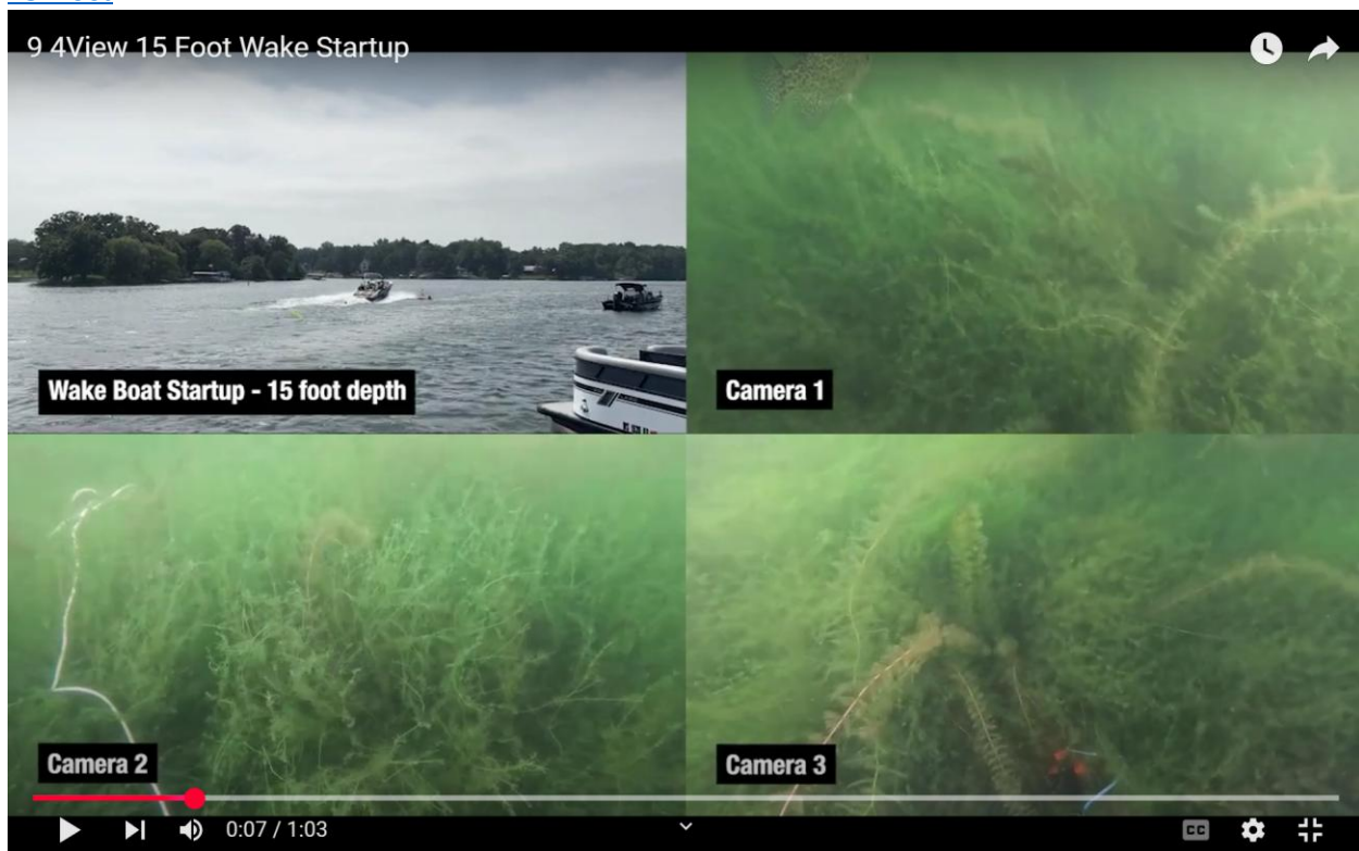
Fig. 12A Phase 3 Subsurface Waves and Propeller Downwash Impacts of Wake Boat Startup at 15 Feet
