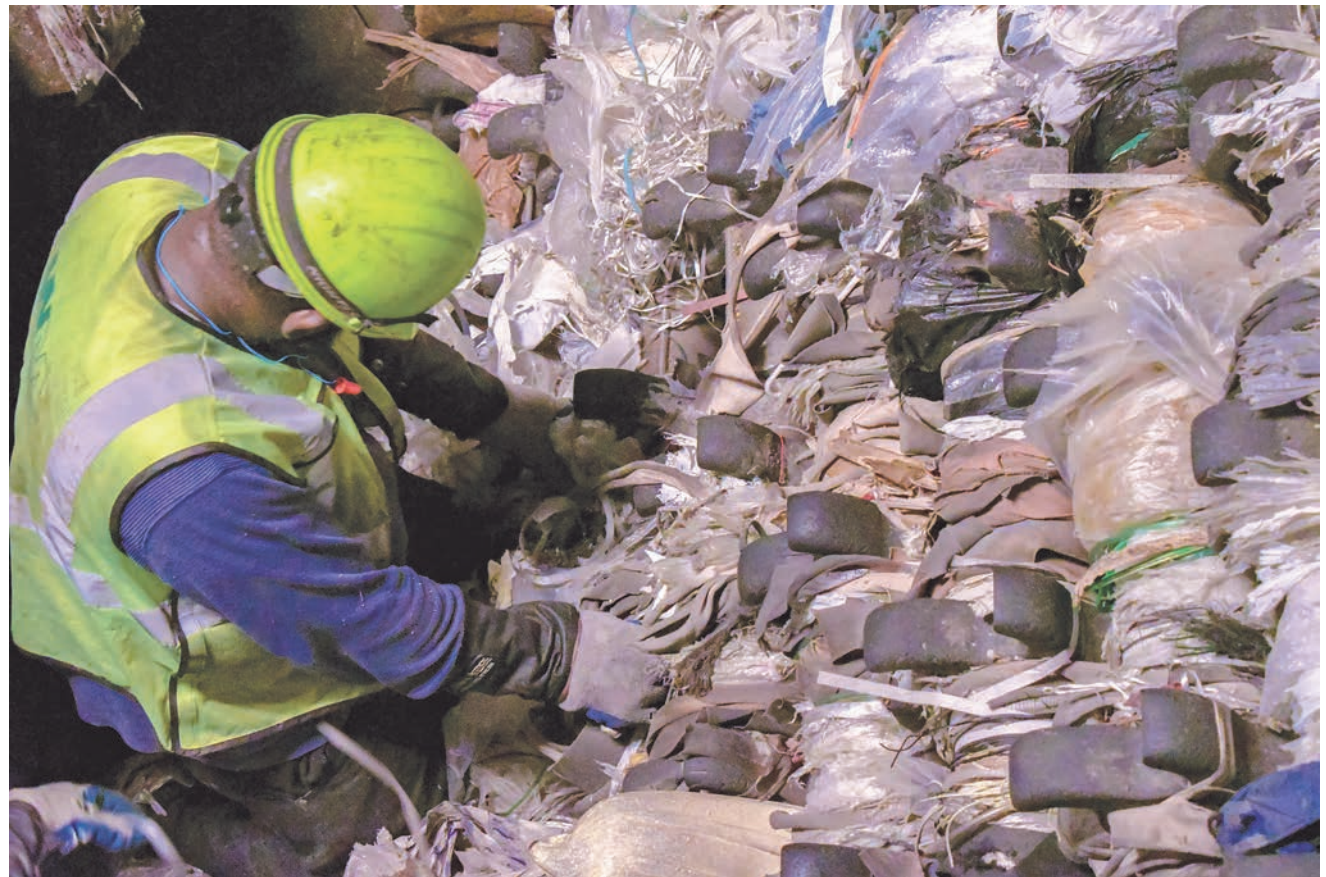
This photo demonstrates one of the problems recycling facilities face when people put undesirable materials in their household recycling bin. In this case, plastic bags, straps, and clothing (referred to as "tangles") have wrapped around processing machinery, rendering it inoperable. Employees must climb onto the machinery to remove the material. Only bottles, cans, jars, jugs, tubs, paper, and cardboard belong in your recycling bins. See the resource table on page 5 to learn about other recycling and waste-related educational resources.
