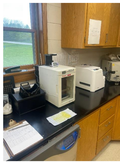
Picture 1.10 – The IDEXX Quanti-Tray Sealer system that was purchased and utilized in 2023 for E. coli testing.
