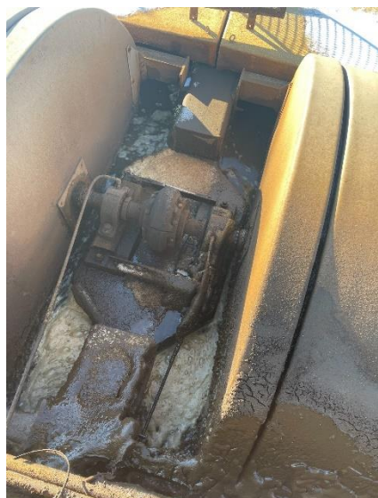
Picture 1.7 – Raptor coupling that has been replaced multiple times in 2023.
