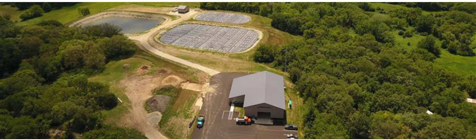
WWTF upgrade, including lagoon aeration improvements and a new administrative building in Palmyra, WI
