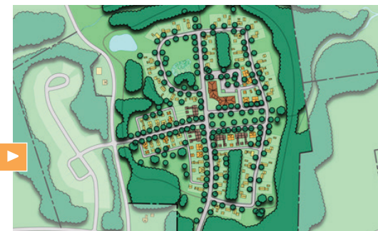
Conservation Design: Increases density of lots while decreasing pavement and length of utilities, while increasing preservation of open spaces and natural areas
