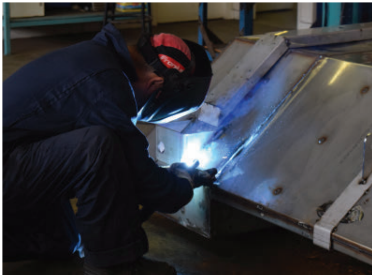
Welding the stainless steel hull has been made easier with the introduction of Fronius welding technology.
