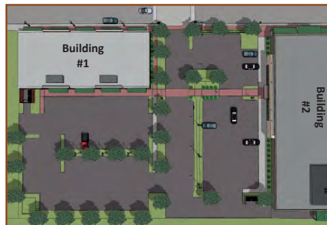
An example of parking being shared between two developments with parking limited to the side or rear yards (no front yard parking).
