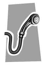
Hand-held shower heads which comply with state regulations for cross connection will have the code **ASME 112.18.1** stamped on the handle. In addition, make sure your hand-held shower head is at least 1 inch above the top of the flood level rim of the tub when it's hanging freely.
