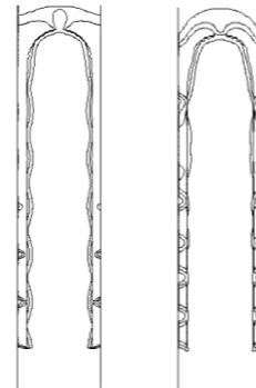
Fig.3 Electric field distribution with contour line (Left : 638nm, Right : 532nm)
