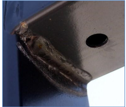
A mild steel weld similarly used on the gate frame. The effect of weld heat on the gal coating is clearly evident. The 'black' weld and damaged gal has begun to rust on this gate installed for less than 12 months.
