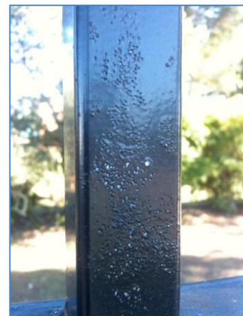
The 'orange peel' is a result of low quality powders and poor pretreatment and cleaning of the product and/ or inferior tube.
