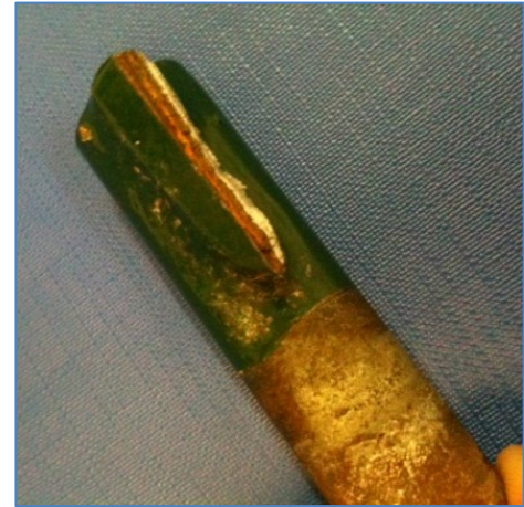
A Goliath hinge that has seized and failed snapping where it affixes to the gate resulting in the gate falling over.
