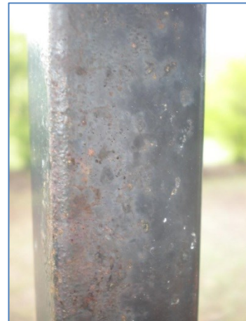
Red rust starting to appear through the powder coating at 3 years.
