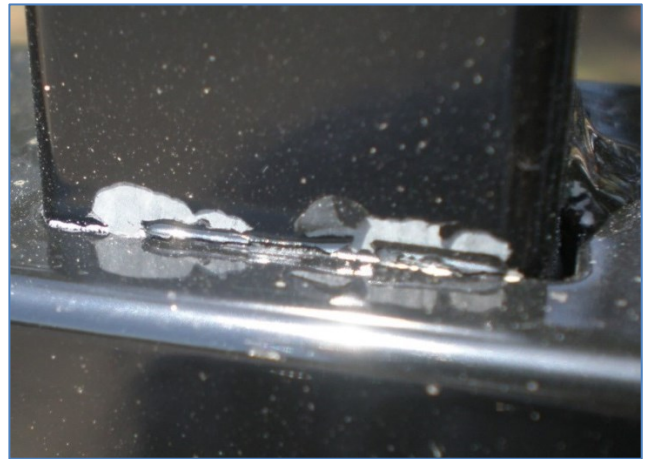
The delamination of the powder film is a result of poor metal pretreatment. Image taken less than 1 month after installation.
