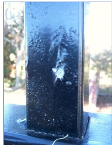
The delamination of the powder film is a result of oxidisation (white rust). Fence installed less than 18 months.
