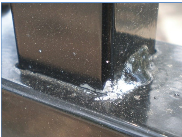
Another image of a mild steel or 'black' weld. This panel had been installed about 1 month.
