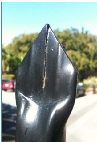
This is an imported panel installed about 15 months. The poor quality tube is brittle resulting in splitting during manufacture and consequent corrosion.
