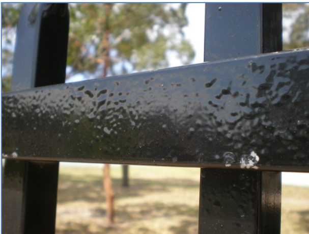
This finish show excess powder has been applied and will have poor adhesion as a result.
