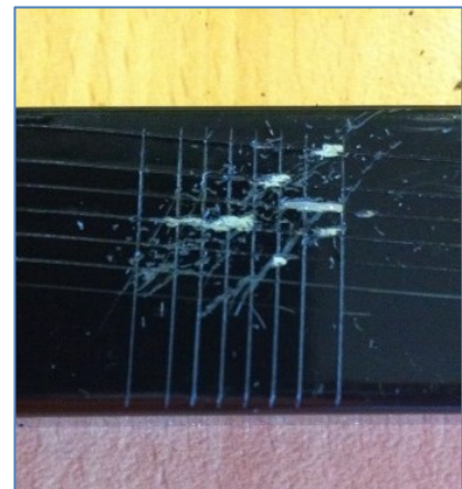
The coating failing the basic cross hatch test under AS4506. A blade creates a cross hatch on the powder surface. The powder sections should adhere when flicked with the edge of the blade. Image of 'new' fence.
