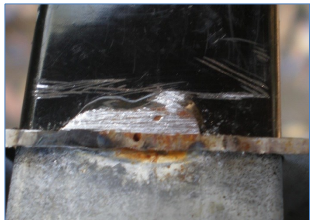
A cut away of a mild steel weld. The effect of weld heat on the gal coating is clearly evident. A silicon bronze weld is cooler so results in less damage to the zinc coating.
