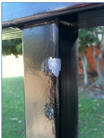
Delamination of the powder film. Proper chemical pretreatment and quality powders cost more.
