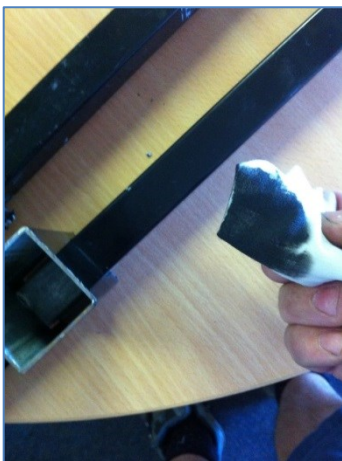
The failure of the coating to pass the basic MEK solvent rub test under AS4506. This indicates poor quality powder, poor metal pretreatment and under cure of the powder. Image of 'new' fence.
