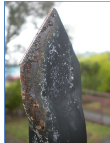
This is an image of a spear in the same section of fencing as the spear (left) some 3 years after installation.
