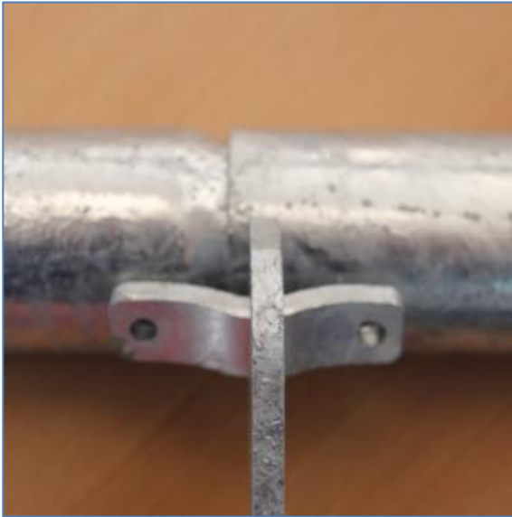
The join in the pieces of swaged rail are positioned over the Standard Bracket so that the U-clip straddles the two.
