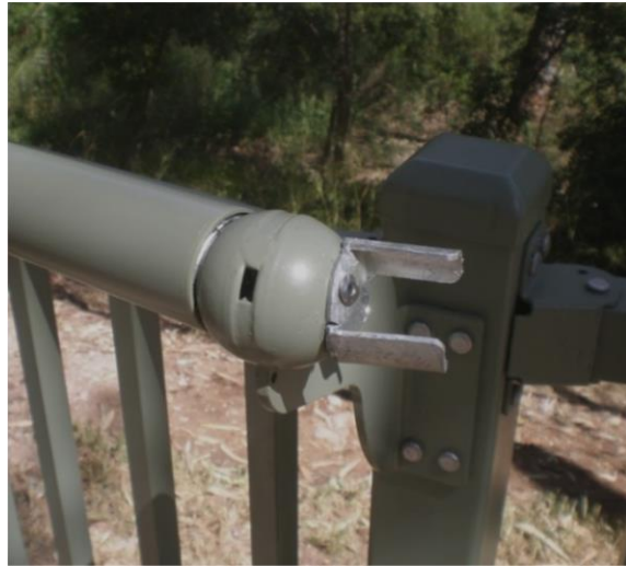
Dome Base fixed to the Ball Bracket with 2 x Ø4.8mm stainless steel rivets.
