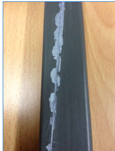
This image shows a sample tube after Neutral Salt Spray (NSS) adhesion test at 1000 hours. There is significant under cut (delamination) off the scribe indicates the coating fails the NSS test under AS4506 at 1000 hours.
