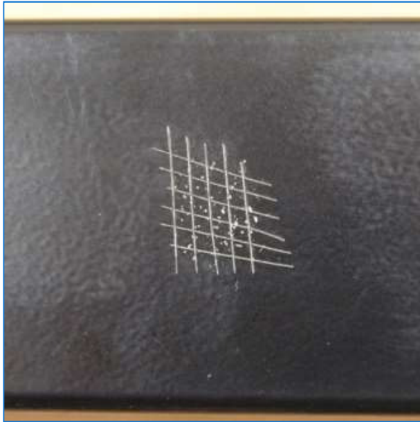
This image shows the cross hatch test of product powder coated by Bluedog. A tool/ blade creates a cross hatch on the powder surface. The powder sections should adhere when flicked with the edge of the blade. The lack of delamination of the square hatches indicates the coating passes the cross hatch test under AS4506.
