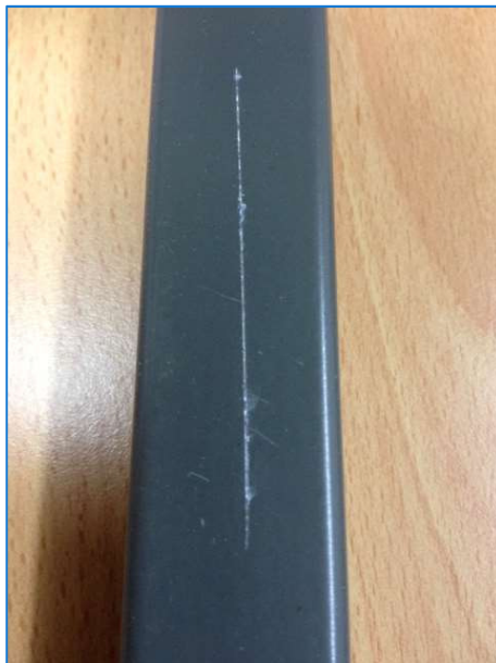
This image shows a Bluedog sample tube after Neutral Salt Spray (NSS) adhesion test at 1000 hours. There is less than 2mm of under cut (delamination) off the scribe indicates the coating passes the NSS test under AS4506.
